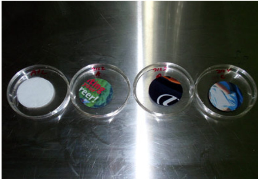
Photograph of samples prior to inoculation with K. pneumoniae ATCC 4352.
